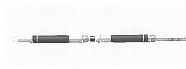
Figure 2 - Example of testing equipment with a double packer (MRPA-Schlumberger)
