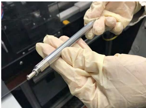
Fig. 2. Test fuel pins of the new chromium coated Zircaloy with new fuel pellets welded inside, developed by Framatome [3]
