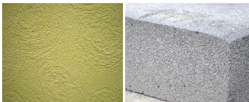
Fig. 1. a) Diatom mud b) Foam concrete
