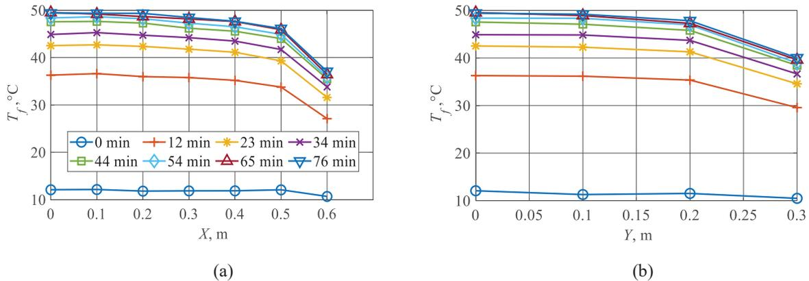
**FIGURE 5.** Temperature distribution of the panel surface at a height of  $Z = 0.75$  m along the coordinate directions X (a), Y (b) at characteristic times
