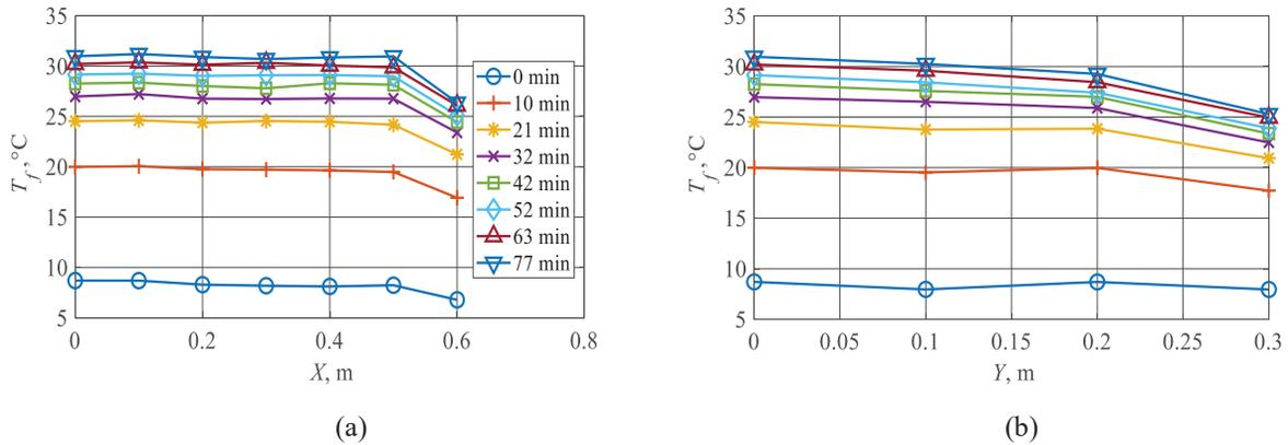
**FIGURE 4.** Temperature distribution of the panel surface at a height of  $Z = 0.75$  m along the coordinate directions X (a), Y (b) at characteristic times
