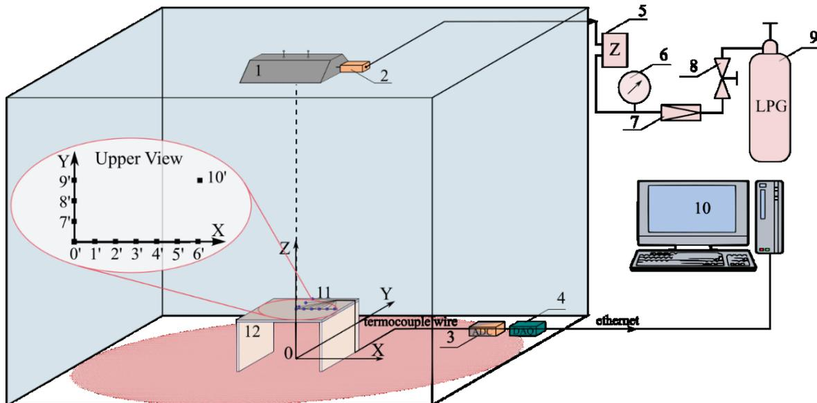
**FIGURE 1.** Schematic representation of the experimental area and the location of thermocouples on the heat supply object model: 1 - GIE, 2 - a GIE control unit, 3 - an analog-to-digital converter, 4 - a data collection system, 5 - a gas flow meter, 6 - a pressure gauge, 7 - a gas pressure regulator, 8 - a main shut-off device, 9 - a gas cylinder, 10 - a computer, 11 - the thermocouples (0' - 10' thermocouple numbers), 12 - a heat supply object
