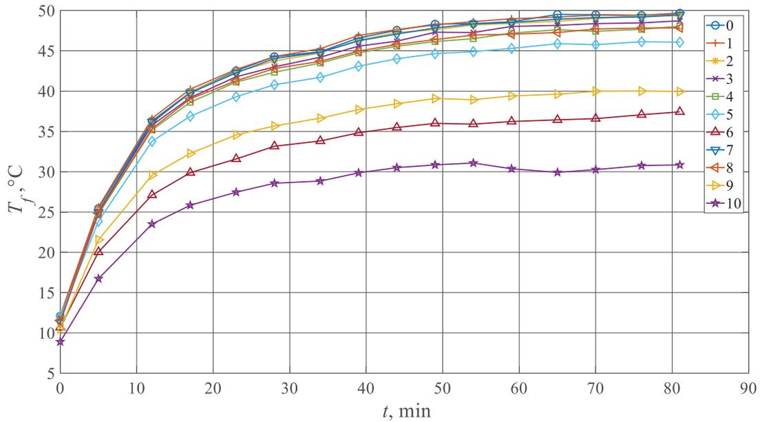
**FIGURE 3.** Temperature changes of the panel surface located at a height of  $Z = 1.5$  m with increasing time (thermocouple numbers according to Table 1)
