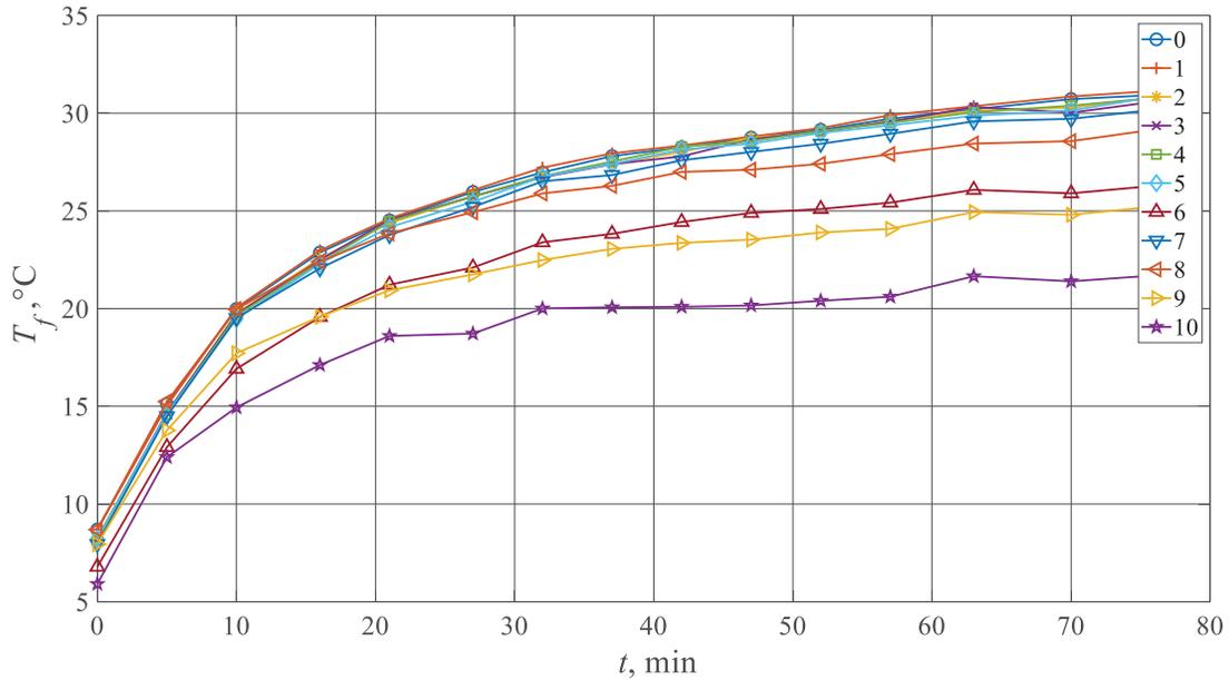
**FIGURE 2.** Temperature changes of the panel surface located at a height of Z = 0.75 m with increasing time (thermocouple numbers according to Table 1)
