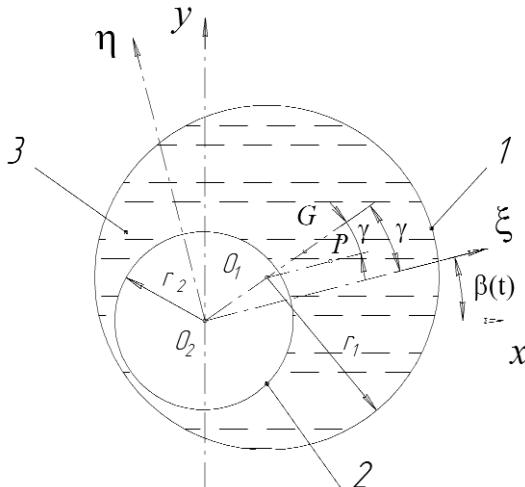
**Figure.** Cross section of rotor with ADL
