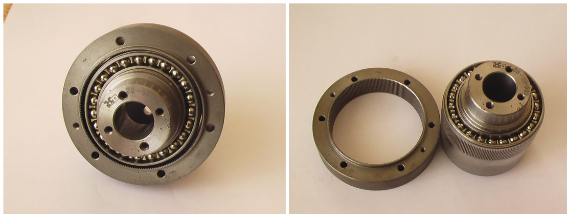
Fig. 1. Wave gear with a flexible spline (on the left it is ready-fitted, on the right static spline is removed)
