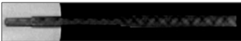
Fig. 3. CT scan data of 3D printed prototype of the FC65-P ionization chamber in 3D printed phantom insert
