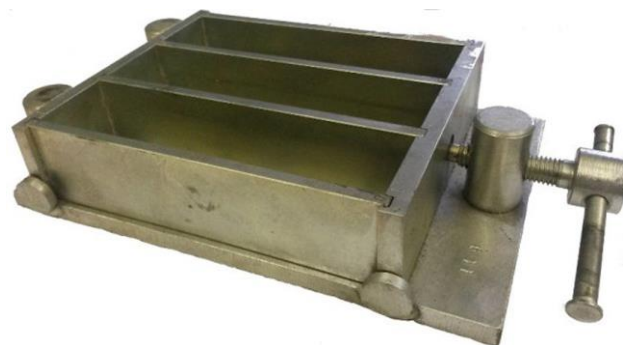
Figure 1. The mould for manufacturing control samples (square section prisms).
