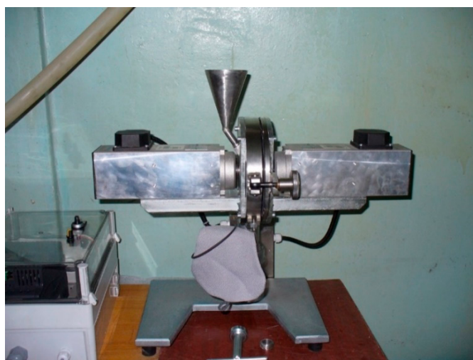
Figure 1. The laboratory installation intended for mechanical activation.
