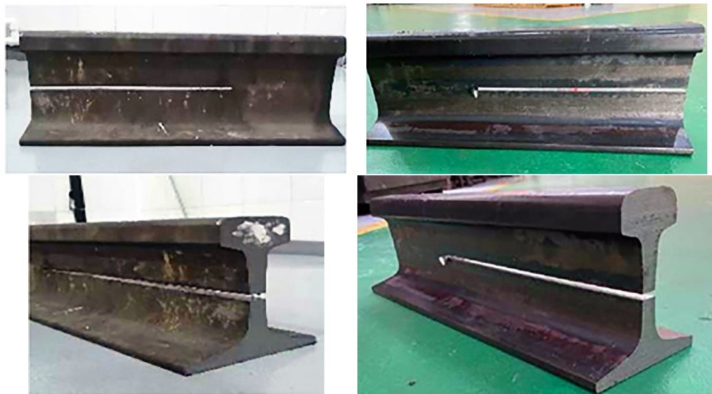
Figure 10. Samples after residual stress control in a rail neck.
