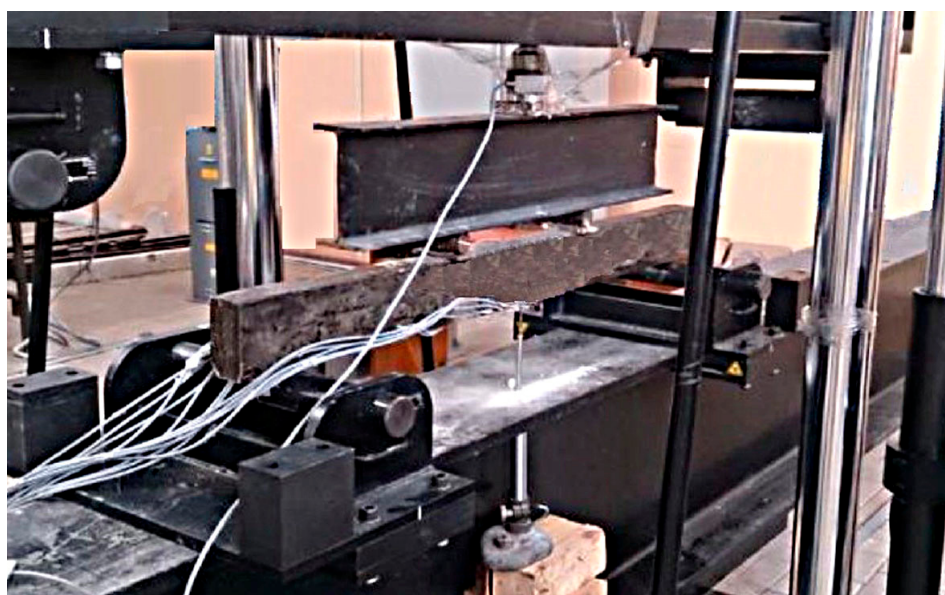
Figure 2. General view of the bending test of rubber concrete beams.
