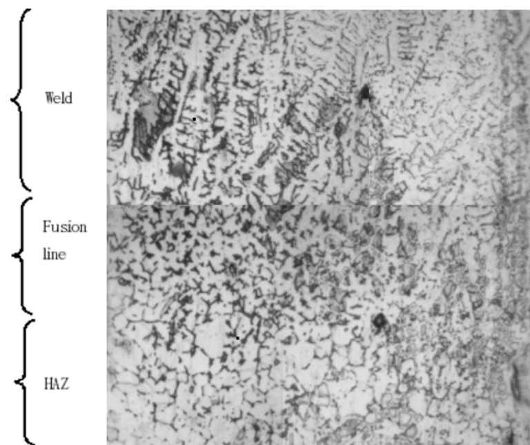
Figure 5. Collage of microstructures of a welded joint made of AISI 316L steel at low values of mode parameters ( \times 500 ).
