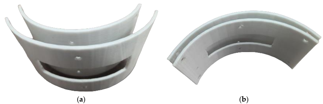
Figure 10. The templates for the flexible acoustic array: (a) the convex; (b) the concave.
