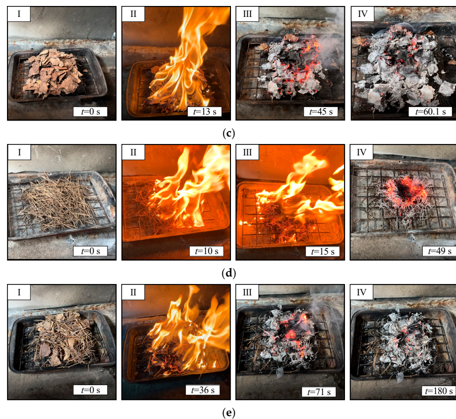
Figure 2. Images of laboratory-scale fires at different combustion stages: I—combustible material sample at the initial point (before ignition); II—active combustion; and III—decay and smoldering; IV—release of combustion products stops. (a)—branches; (b)—timber; (c)—leaves; (d)—needles; and (e)—mixture of forest fuels.
