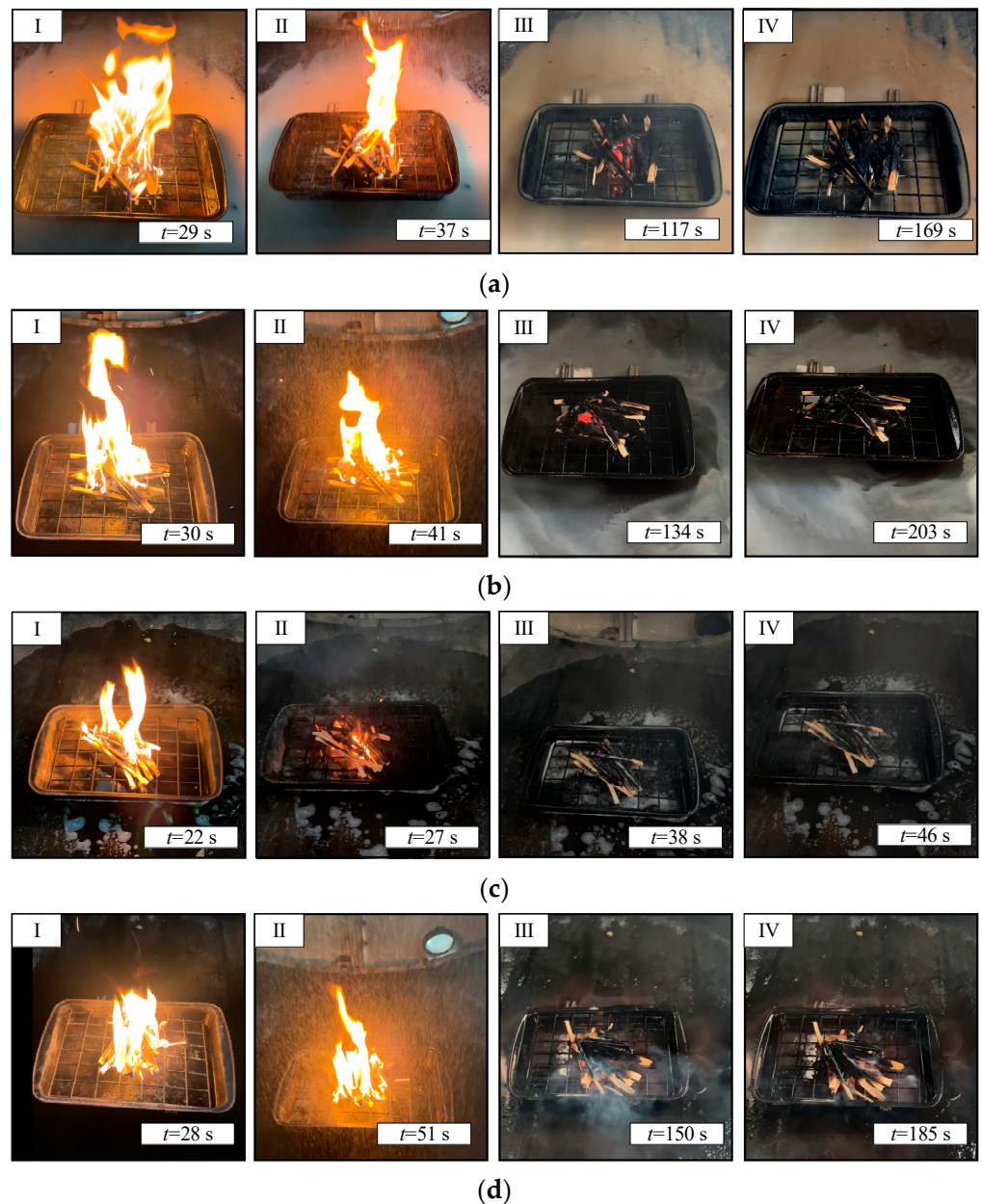
Figure 4. Images of laboratory-scale fires under investigation at different combustion and suppression stages: I—active combustion; II—suppression; III—smoldering; and IV—completion of combustion product release: (a)—bentonite; (b)—bischofite; (c)—foaming agent; and (d)—water.
