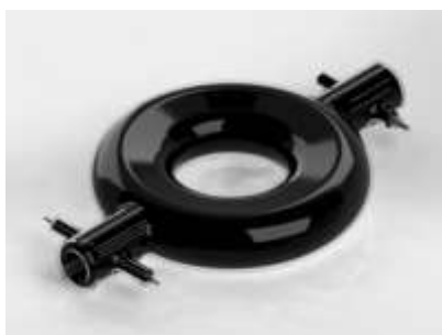
Figure 1. Sealed vacuum acceleration chamber of 6 MeV betatron.
