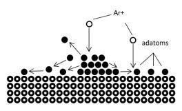
Figure 3. Scheme of Ar ion interaction with the surface
