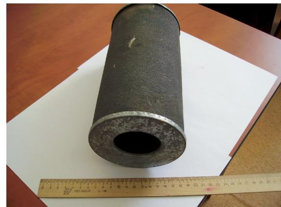
**Fig. 9.** Filter element of diesel oil filter
