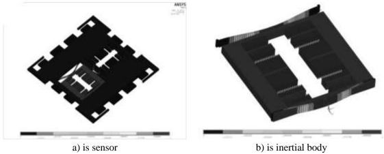
**Figure 3.** The first mode of sensor eigenfrequencies ( $f_v = 5032.57 \text{ Hz}$ ).
