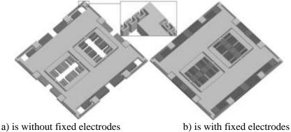
Figure 2. MMG Silicon sensor.
