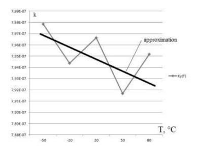
**Figure 10.** Dependence of scale factor vs temperature.
