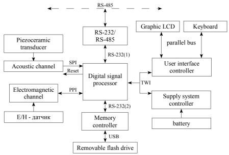
Figure 1. Block diagram of the recorder.
