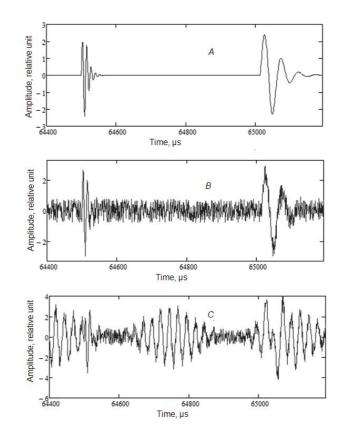
Figure 3. Informative electromagnetic signals of 20 kHz and 80 kHz (a); the same signals with white noise (b) white noise and sinusoidal electromagnetic interference (c).
