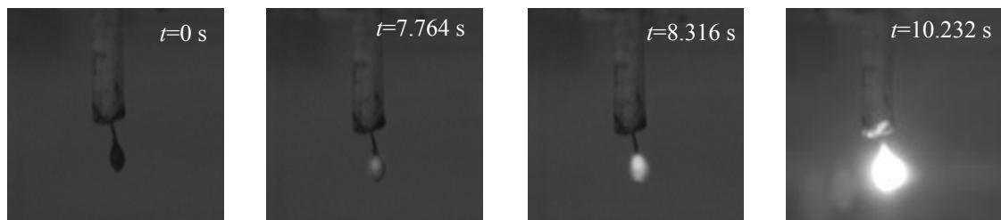
Fig. 2. The ignition of a coal-water slurry fuel droplet, the composition No. 1, T_a=550 °C.
