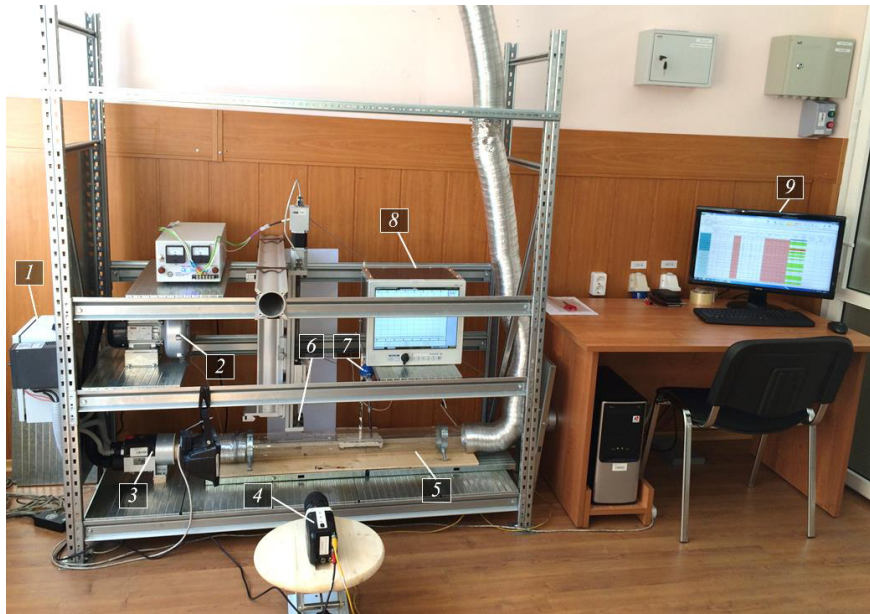
Fig. 1. Experimental setup: 1 – heating system remote control; 2 – high-pressure blower; 3 – air heater; 4 – high-speed video camera; 5 – hollow glass cylinder; 6 – positioning mechanism for droplet supply; 7 – thermocouple; 8 – multichannel registrar; 9 – computer.
