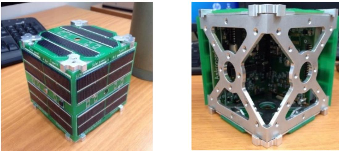
*Fig. 1. Nano-satellite equipped with solar panels*
