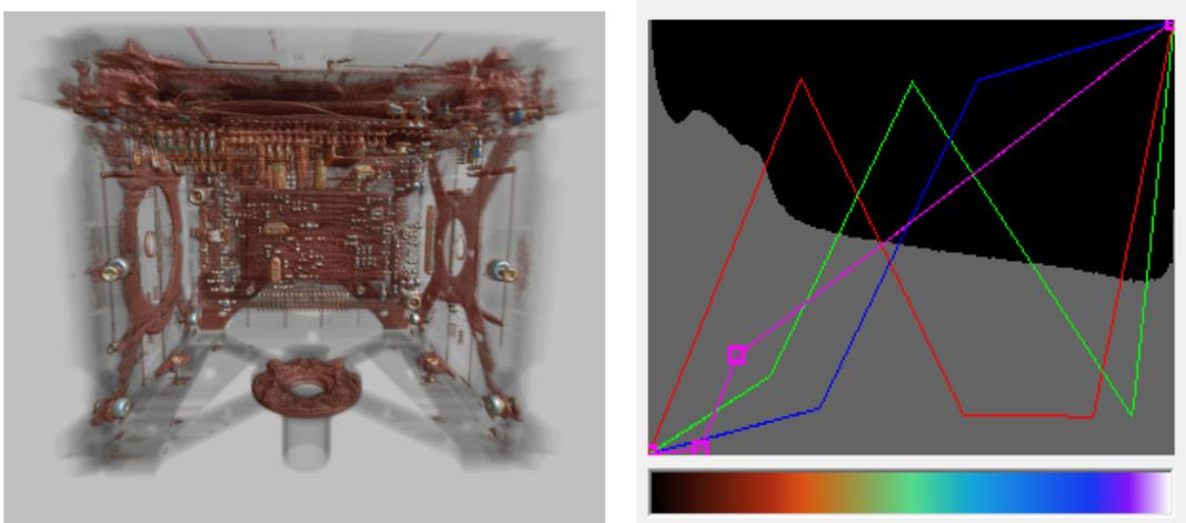
*Fig. 2. X-ray micro tomography of a nano satellite:
