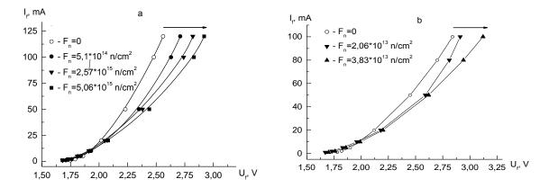
**Figure 2.** Volt-ampere characteristic of LED produced on the base of AlGaInP heterostructures with multiple quantum wells irradiated by fast neutrons: a) – LED ( $\lambda$ =623 nm); b) – LED ( $\lambda$ =590 nm); symbols – measurement results; lines – identified regularities; arrows indicate the direction of changing volt-ampere characteristics
