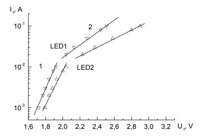
**Figure 1.** Volt-ampere characteristic of LED in semilogarithmic scale: 1 – mid-level injection zone; 2 – high injection zone; symbols – results of measurement; lines – identified regularities
