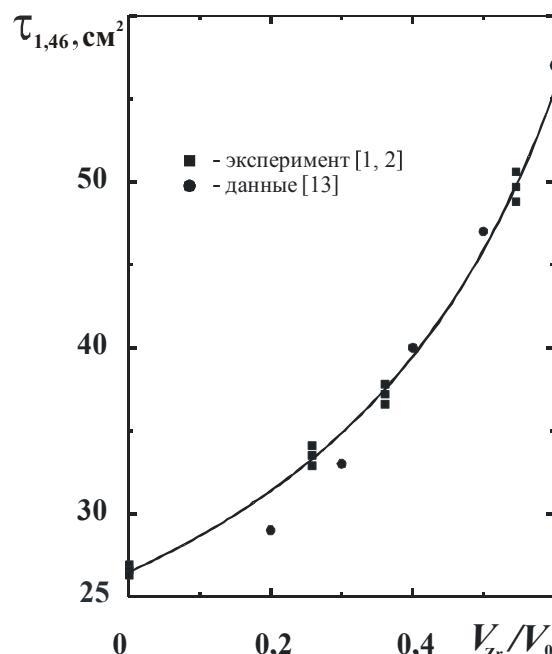
Fig. 2. The experimental data approximation by fission neutron age by [1, 2] for the mixture  $\text{Zr}-\text{H}_2\text{O}$ , eq. (3)
