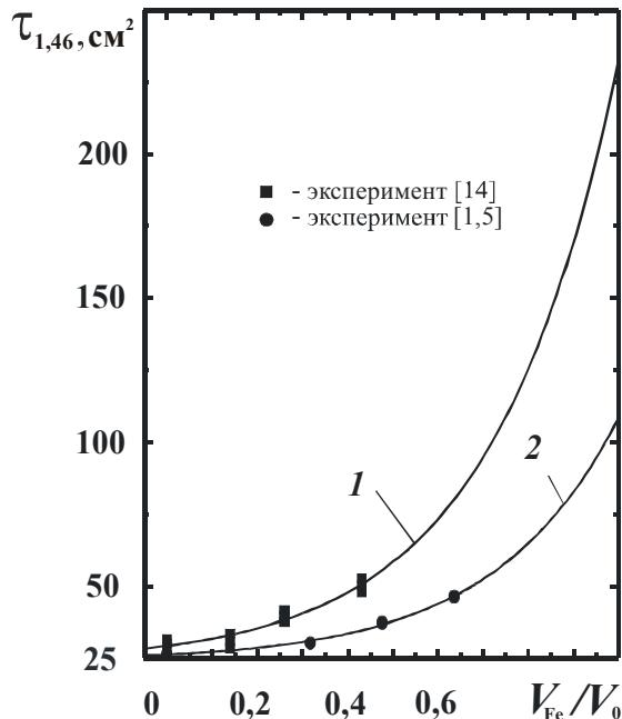
**Fig. 4.** Test data approximation by age in  $\text{Fe}-\text{H}_2\text{O}$  mixtures: 1) by eq. (6), 2) by eq. (7)
