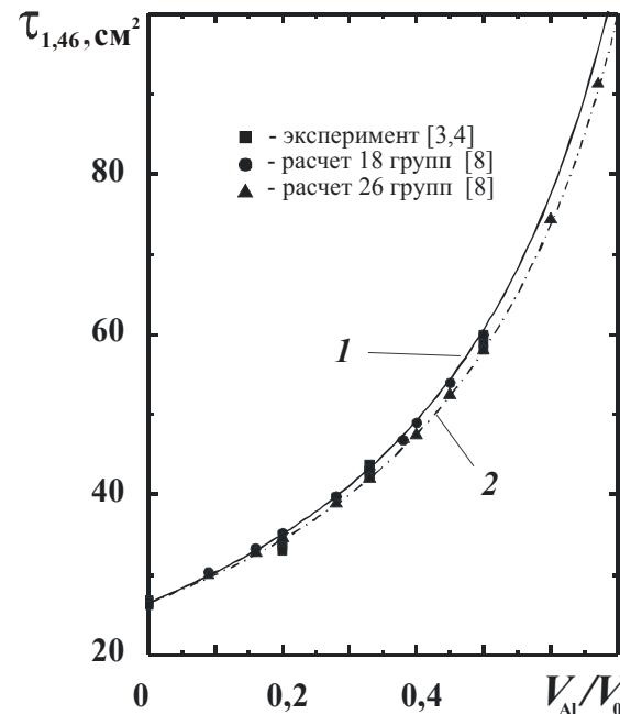
Fig. 3. Dependence of fission neutron age on metal part in the mixture  $\text{Al}-\text{H}_2\text{O}$ : 1) by eq. (4), 2) by eq. (5)
