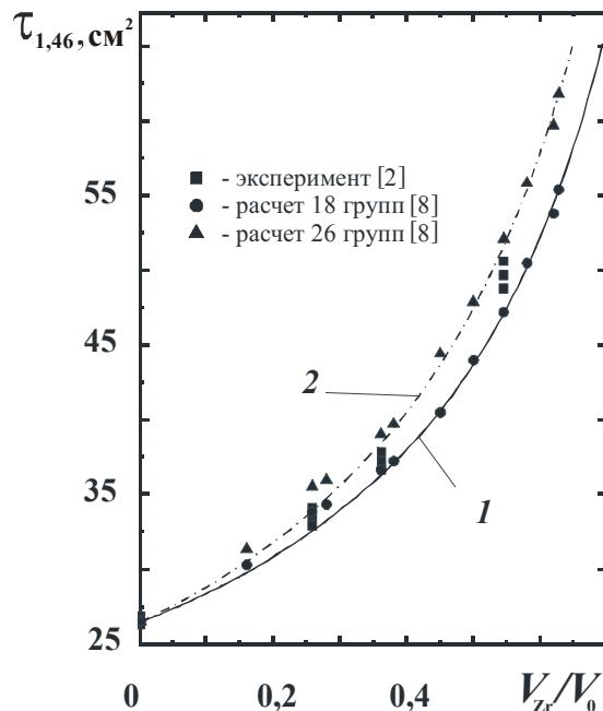
Fig. 1. Dependence of fission neutron age on metal part in the mixture  $\text{Zr}-\text{H}_2\text{O}$ : 1) by eq. (1); 2) by eq. (2)
