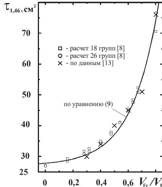
**Fig. 6.** Age matching of rated data in the mixture  $\text{Fe}-\text{H}_2\text{O}$  with the data [13]
