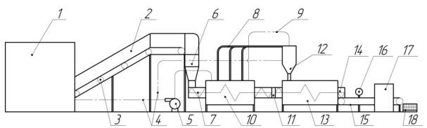
**Figure 1.** Layout diagram of the process line at small-tonnage solid composite fuel production: 1 – storeroom, 2 – dry of raw, 3 – conveyer, 4 – conduit of flue gases, 5 – exhauster, 6 – grinder, 7 – conveyer screw, 8 – conduit of volatile products, 9 – conduit of gas, 10 – combustion chamber, 11 – box-coupling, 12 – unit of binder preparation, 13 – heat-exchange unit, 14 – conveyer screw, 15 – conveyer, 16 – press roll, 17 – molder of stamping, 18 – dilly.
