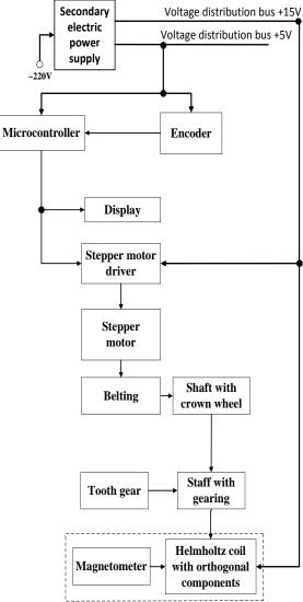
Fig. 1. Functional diagram of the automatic calibration of deep-water magnetometer
