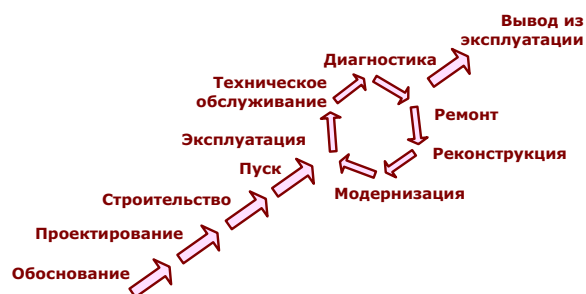
Fig. 1. Stages of the equipment unit lifecycle
