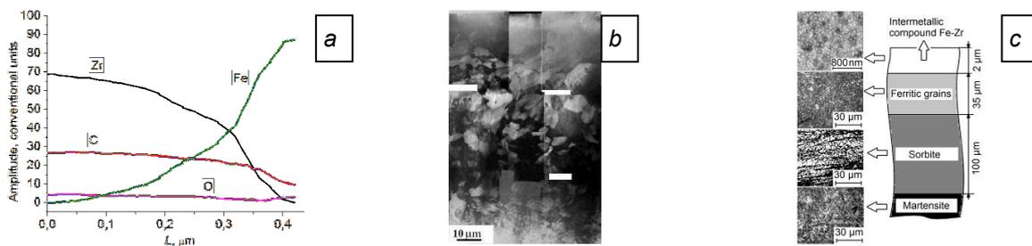
Fig. 1. Dependence of chemical elements concentration through the surface layer depth (a); TEM image of the subsurface layer cross section of the specimen after the irradiation (b); layered macrostructure scheme (c)
