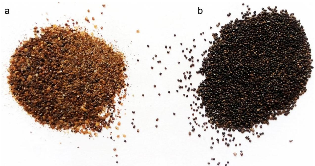
Figure 6 – Iron ore after magnetic separation:
