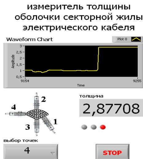
Fig.9. The front panel
