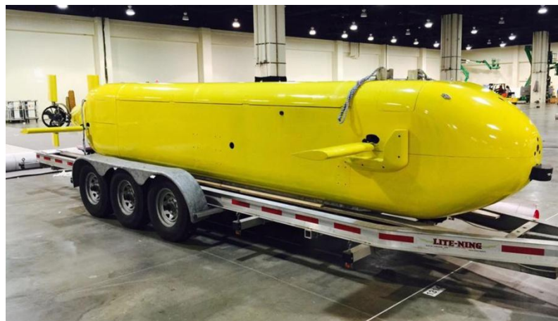
Fig. 1.4 – AUV “LDUUV” of US Navy equipped with control blades
