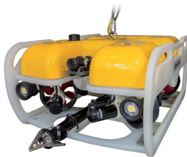
Fig. 1.1 – Remotely operated UUV “Marlin-350” equipped with a manipulator
