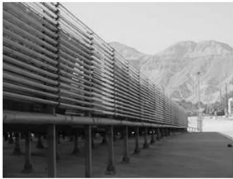
Figure 1.4 - Open circulating systems for the cultivation of chlorella
