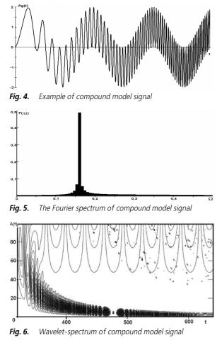
Only one clearly defined harmonic characterising modulated periodic signal is evident from the Fourierspectrum. To judge the presence of the second modelling
