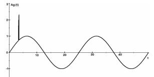
**Fig. 1.** Example of periodic signal with the surge at positive half-period
