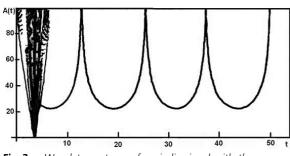
Fig. 3. Wavelet-spectrum of periodic signal with the surge at positive half-period
