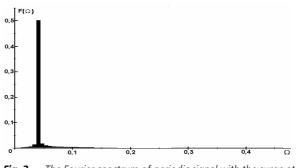
Fig. 2. The Fourier spectrum of periodic signal with the surge at positive half-period
