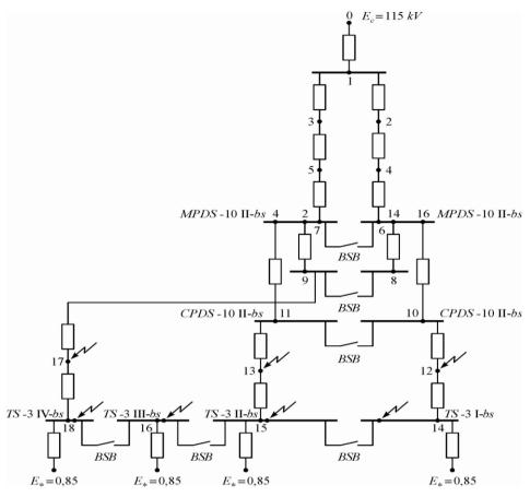
Figure 1. Equivalent circuit of power supply of part of sublimation plant
