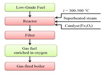
**Figure 1.** Heat processing of low-grade fuel.
