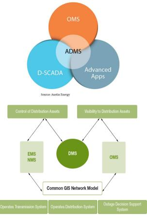
Figure 1. The structure of distribution management system.
