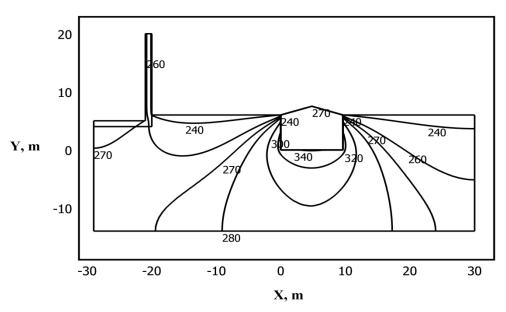
Figure 3. Typical temperature field in the zone of the storage tanks for fuel thermal power plants and boiler at ambient temperature -40 °C, taking into account the impact of engineering structures.
