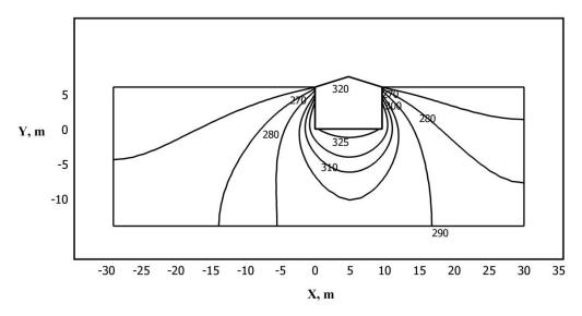
Figure 2. Typical temperature field in the zone of the storage tanks for fuel thermal power plants and boiler at ambient temperature -40 °C.
