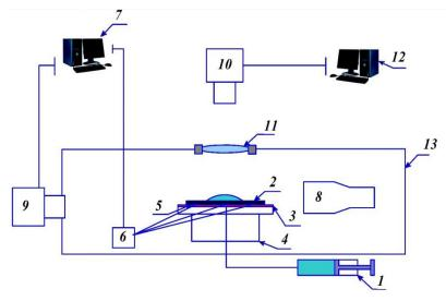
**Fig. 1.** The scheme of the experimental setup: 1 – syringe pump; 2 – substrate; 3 – thermoelectric module; 4 – goniometer; 5 – thermocouples; 6 – analog-to-digital converter; 7, 12 – personal computers; 8 – light source; 9, 10 – high-speed video cameras; 11 – lens of the upper optical system; 13 – transparent box.
