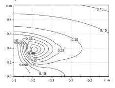
Fig. 9. The distribution of the mass concentration of carbon monoxide.
