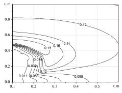
**Fig. 7.** The distribution of the mass concentration of carbon monoxide ( $C_{10}=0.1$ ,  $\Delta P=2\cdot 10^3$  Pa).
