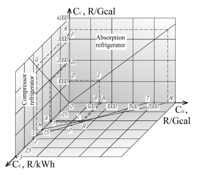
**Fig. 1.** Dependence of refrigeration cost price on heat and electric energy cost price in the system of trigeneration.
