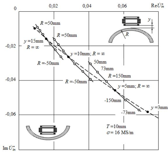
**Figure 4.** Hodographs of the relative induced SECP voltage for the change in the gap and the radius of the test object surface curvature.
