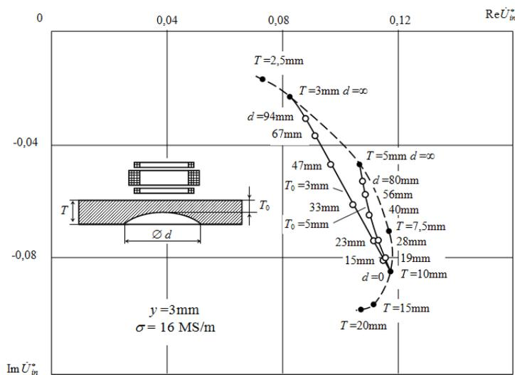
**Figure 7.** Hodographs of the SECP relative voltage for the change in the diameter of the spherically-shaped local thinning.
