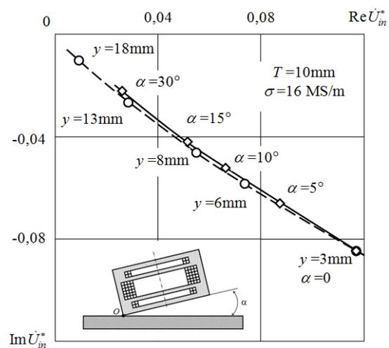
**Figure 6.** Hodographs of the SECP relative induced voltage for the change in the skew angle  $\alpha$ .
