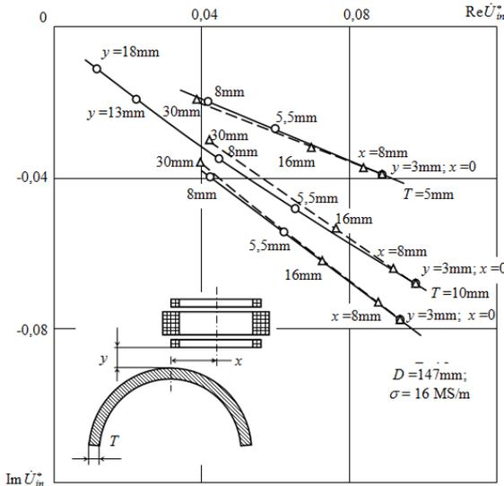
**Figure 5.** Hodographs of the relative induced SECP voltage for the longitudinal axis with respect to the pipe transverse axis.
