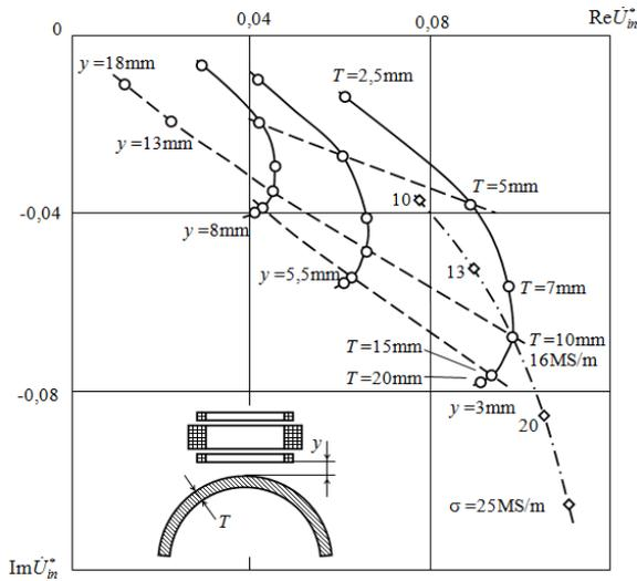
**Figure 3.** Hodographs of the relative induced SECP voltage for the change in the pipe wall thickness  $T$ , the gap  $y$  and the material conductivity  $\sigma$ .
