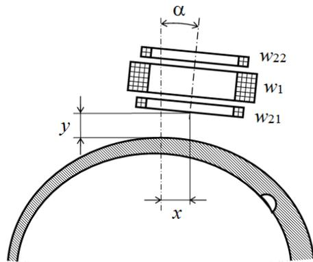
**Figure 1.** SECP interacting with the conductive pipe.
