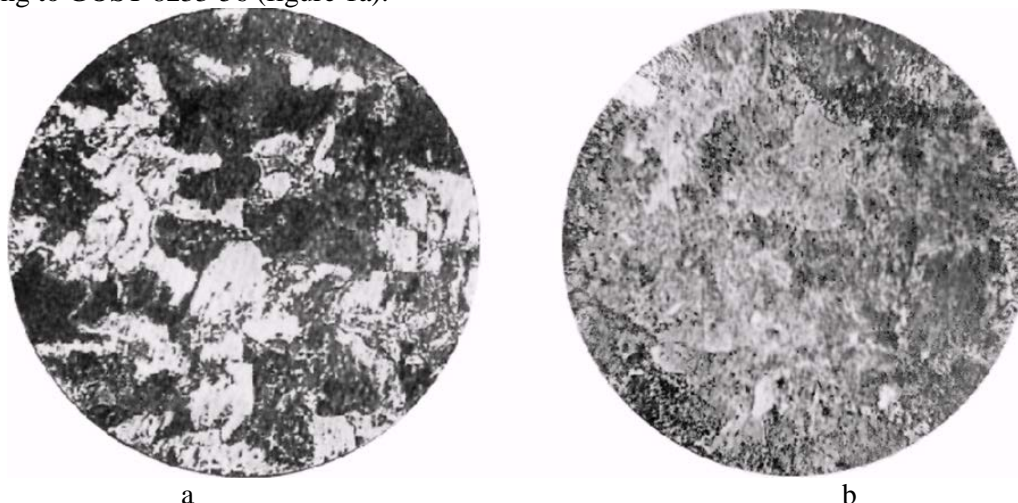
Figure 1. Photo-standards of lamellar pearlite GOST 8233: a – grade 1, b – grade 2.
