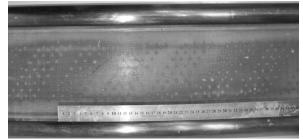
**Figure 2.** Ion beam autograph left on the emission grid on the side of the high-voltage acceleration gap in the experiment with no mask in the emitter.
