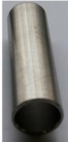
**Figure 5.** Samples before ion polishing ( $\varnothing 9.15$  mm)
