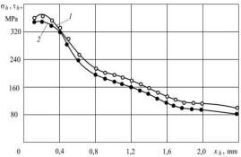
**Figure 3.** Distribution of normal  $\sigma_h$  ( $\circ$ ) and tangential  $\tau_h$  ( $\bullet$ ) contact loads over the flank-land of the cutter in cutting of the brittle brass (57Cu1Al3Mn).  $\gamma = 0^{\circ}$ ,  $\alpha = 18^{\circ}$ ,  $\alpha_h = 0^{\circ}$ ,  $\nu = 1.7$  m/s, f =0.41 mm/r. Ordinate – normal  $\sigma_h$  [MPa], and tangential  $\tau_h$  [MPa] specific contact load on the flank-land; abscissa – distance from the cutting edge on the surface of flank-land  $x_h$  [mm]
