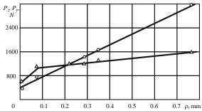
**Figure 8.** Dependence of cutting force component acting on the rake surface  $P_{Yr} \ \mu P_{Zr}$  on radius of cutting edge rounding  $\rho$  in titanium alloy BT3-1 machining. BT3-1 – BK8,  $\gamma = 0^\circ$ ,  $\alpha = 10^\circ$ , v = 1 m/s, f = 0.21 mm/r;  $\circ -P_{Yr}[N]$ ,  $\Delta -P_{Zr}[N]$ ; machined disk width b=2.3 mm
