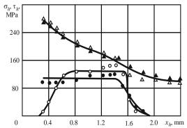
**Figure 4.** Distribution of contact loads over the flank-land of the cutter in brass machining by the cutter with rounding off cutting edge with radius  $\rho = 0.3$  mm.  $\gamma = 0^{\circ}$ ,  $\alpha = 18^{\circ}$ ,  $\alpha_h = 0^{\circ}$ , v = 1.7 m/s,  $\circ$ , • – ductile brass (63Cu), f = 0.21 mm/r;  $\Delta$ , • – brittle brass (57Cu1Al3Mn); f = 0.41 mm/r;  $\circ$ ,  $\Delta$  – normal contact load  $\sigma_h$ ; •, • – tangential contact load  $\tau_h$
