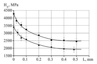
**Figure 3**. Depthward distribution of micro-hardness after ultrasonic treatment:
