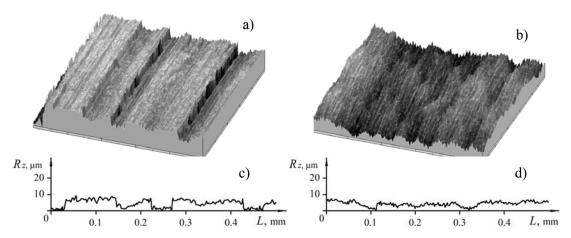
**Figure 5.** 3D-image of the surface (a, b) and profilogram (c, d) after pre-turning: a, c - Steel 20; b, d - steel 40X
