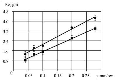
**Figure 9**. Influence of the supply amount of the indenter to a height of asperities after ultrasonic treatment: • - Steel 20; ■ - Steel 40X. Processing velocity 23
