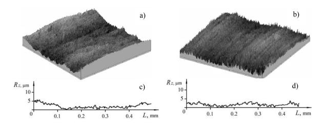
**Figure 7**. 3D-image of the surface (a, b) and profilogram (c, d) after preturning: a, c - Steel 20; b, d - steel 40X
