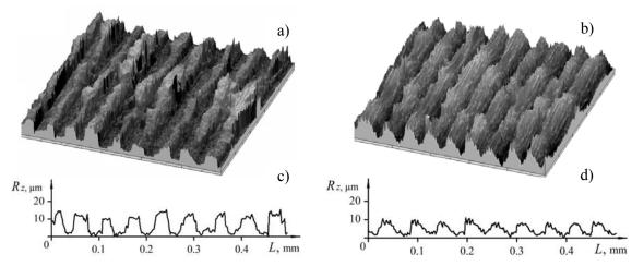
**Figure 4**. 3D-image of the surface (a, b) and profilogram (c, d) after preturning:
