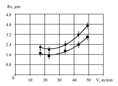
**Figure 10**. Effect of workpiece rotation velocity on micro-roughness heights after ultrasonic treatment: • - Steel 20; ■ - Steel 40X. Indenter feed 0.1 mm/rev
