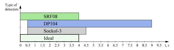
Figure 4. Detection areas of motion sensors and experimental conditions.
