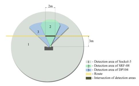
Figure 3. Detection areas of motion sensors and experimental conditions.
