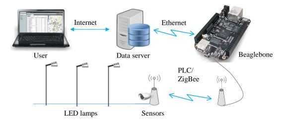
Figure 1. Smart lightning system structure.
