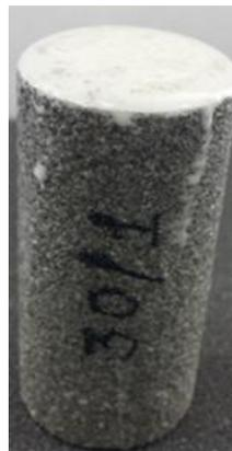
**Figure 5.** Photograph of a core sample with the mud cake after the acid treatment.
