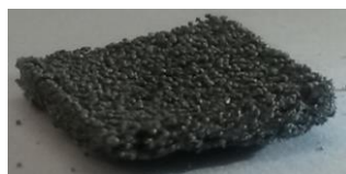
Figure 12. Physical configuration of a three-dimensional sample (x2). Process conditions of sintering: V=1000 mm/min, t=26 °C, S=0.1 mm, P=60 W, increment thickness of layers 200 \mu\text{m} , sintering in argon
