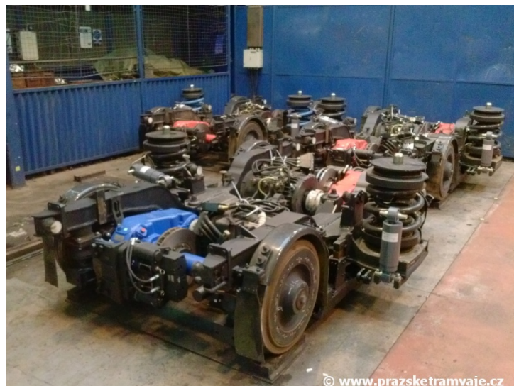
Picture 11 - 14T boogie with primary and secondary springing (Photo: Prazsketramvaje.cz)
