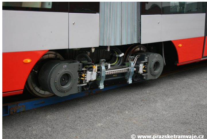
Picture 12 - Detail of connection between wheel and motors (Source: Prazsketramvaje.cz)
