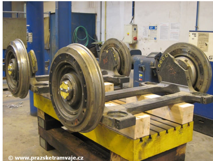
Picture 13 - Boogie of 15T without motors, springing and other features (Source: Prazsketramvaje.cz)
