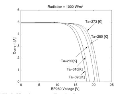
Figure 2- Effects of temperature on silicon solar cells [3]
