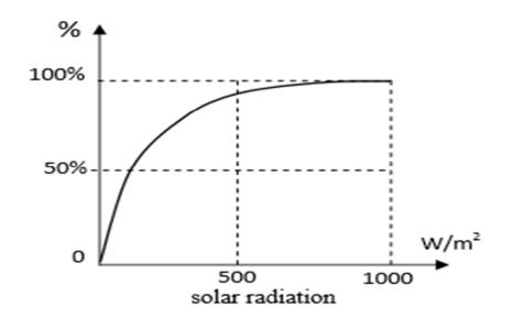
Figure 3- Efficiency dependence of photoconversion on solar radiation [6]
