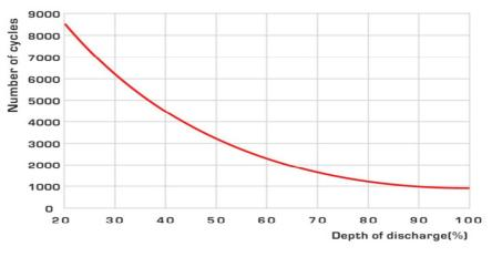
Typical cycle life versus DOD(20 $^{\circ}$ C)
