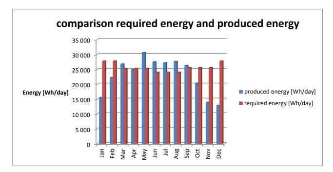
Figure 16- Comparison required energy and produced energy
