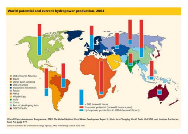
Picture 2- World potential and current hydropower production [2]
