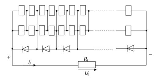
Figure 4- Bypass diodes connection circuit
