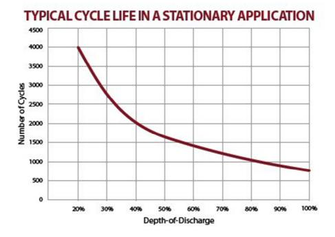
Figure 6- Depth of discharge of lithium- sulphur battery [8]
